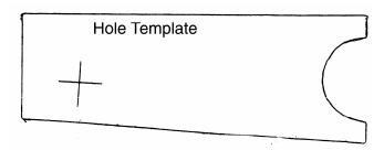
Place the template on the clutch release arm with the bottom edge aligned with the bottom edge of the release arm and the circular part butted against the shaft. Take a center punch and punch the cross in the center to mark the release arm. Drill a 5/16ths hole completely through both sides of the release arm.
